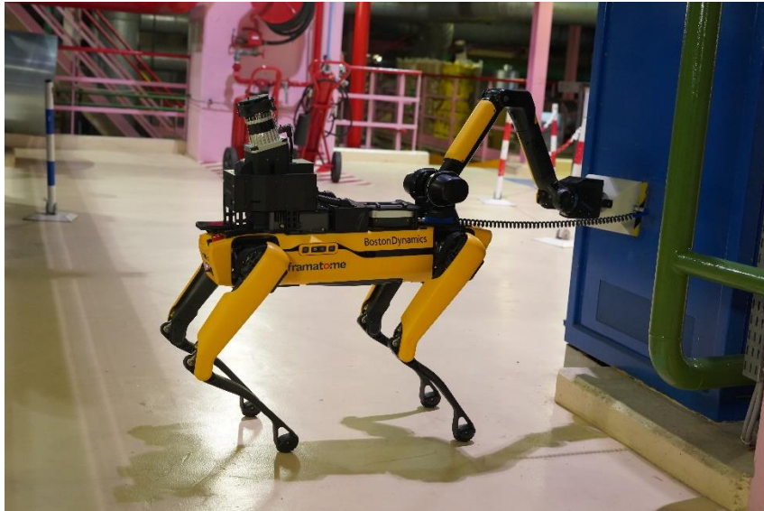
Figure 1 : AMORAC measuring a wall for contamination characterization
