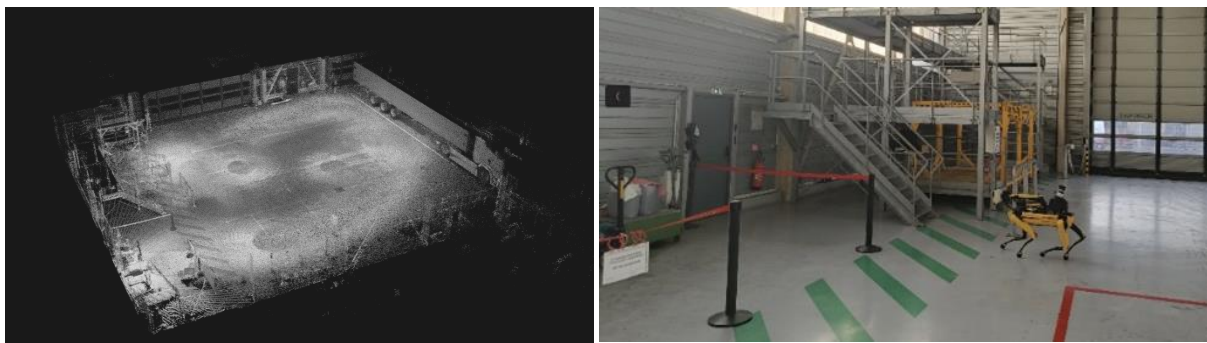
Figure 3 : 3D point cloud of the buffer area for clearance for automated clearance with AMORAC
