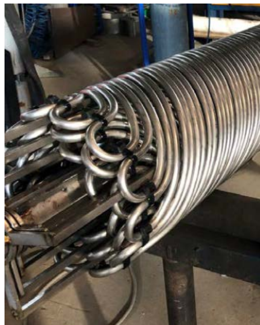
Figure 6 - Close-up of a helical coil steam generator for liquid metals.
