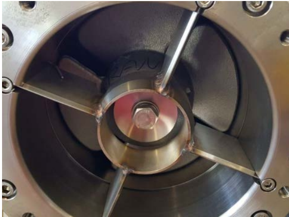
Figure 8 - Prototypical pump impeller for lead coolant.
