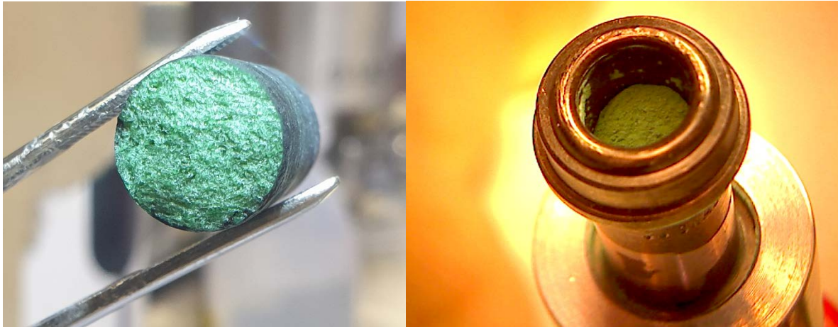
Figure 13: (left) LiF-ThF 4 -UF 4 -PuF 3 salt synthesized at JRC Karlsruhe for the SALIENT-03 irradiation experiment (source: JRC Karlsruhe), and (right) LiF-BeF 2 -UF 4 salt prepared by CV Rez for the SAGA gamma irradiation.
