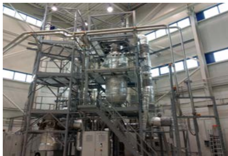
Figure 16: The S-ALLEGRO integral facility (GFR mock-up)
