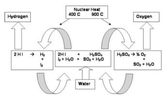
Figure 15 : the sulfur-iodine thermochemical cycle for hydrogen production
