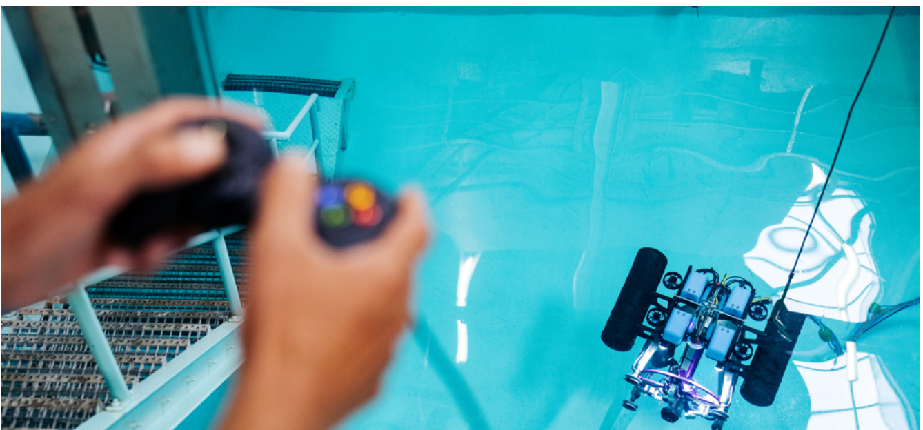
Remote controlled inspection robot Photo: NRG (2020)
