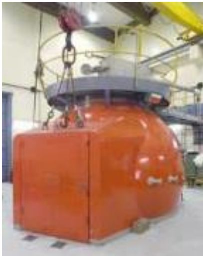
Figure 12 - The TAPIRO fast-spectrum calibration pile.
