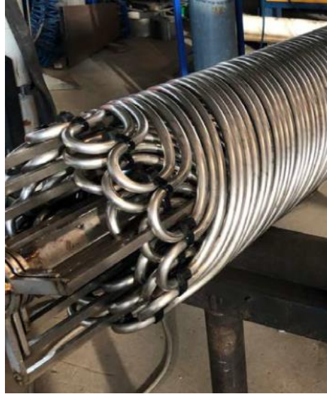
Figure 7 - Close-up of a helical coil steam generator for liquid metals.
