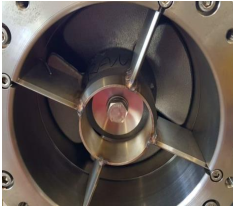
Figure 8 - Prototypical pump impeller for lead coolant.
