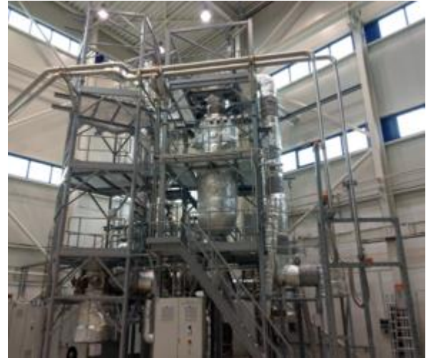
Figure 13: The S-ALLEGRO integral facility (GFR mock-up)
