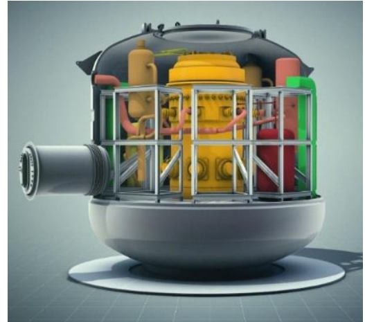
Figure 6-1: NUWARDTM small modular reactor (@TechnicAtome).
