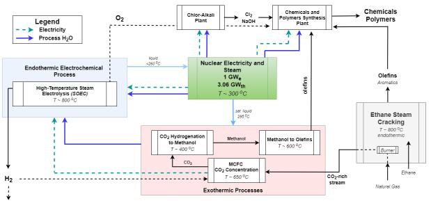
Specific Industrial Park Concept using nuclear heat and electricity to produce chemicals and polymers with minimal CO<sub>2</sub> emissions
