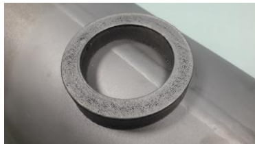
Addition of cylindrical shape 316L, OPTOMECS LENS system
