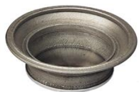
CEA-Gerailp, Inco718 near shape casing
