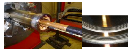
CEA-DEN/Nutech Colmonoy52 Inner Cladding of Tubes
