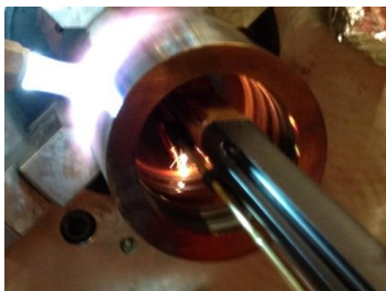
Clading of internal surface of tube diam.100mmx500mm
