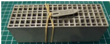
Alexandre type specimen for tensile test
