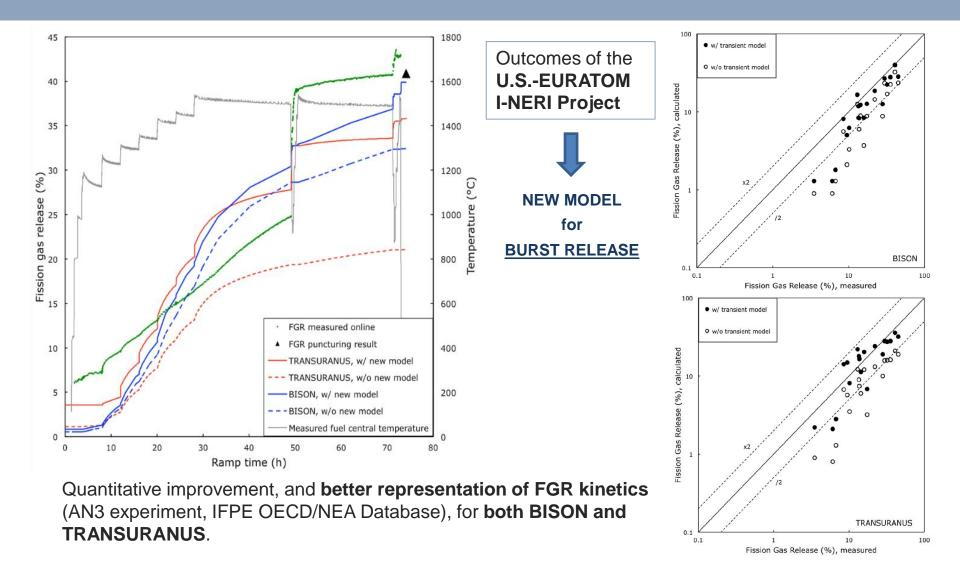
Barani et al., Analysis of transient fission gas behaviour in oxide fuel using BISON and TRANSURANUS, JNM 491 (2017), 55–66.
