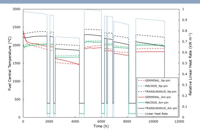
**Different temperature** regimes and evolution, as a function of irradiation, predicted by the codes, especially in the first cycles. This can be ascribed both to the **different gap sizes**, thus to the different gap conductance and radial relocation models (subject to large uncertainties), and to the different fuel thermal conductivity correlations employed.
