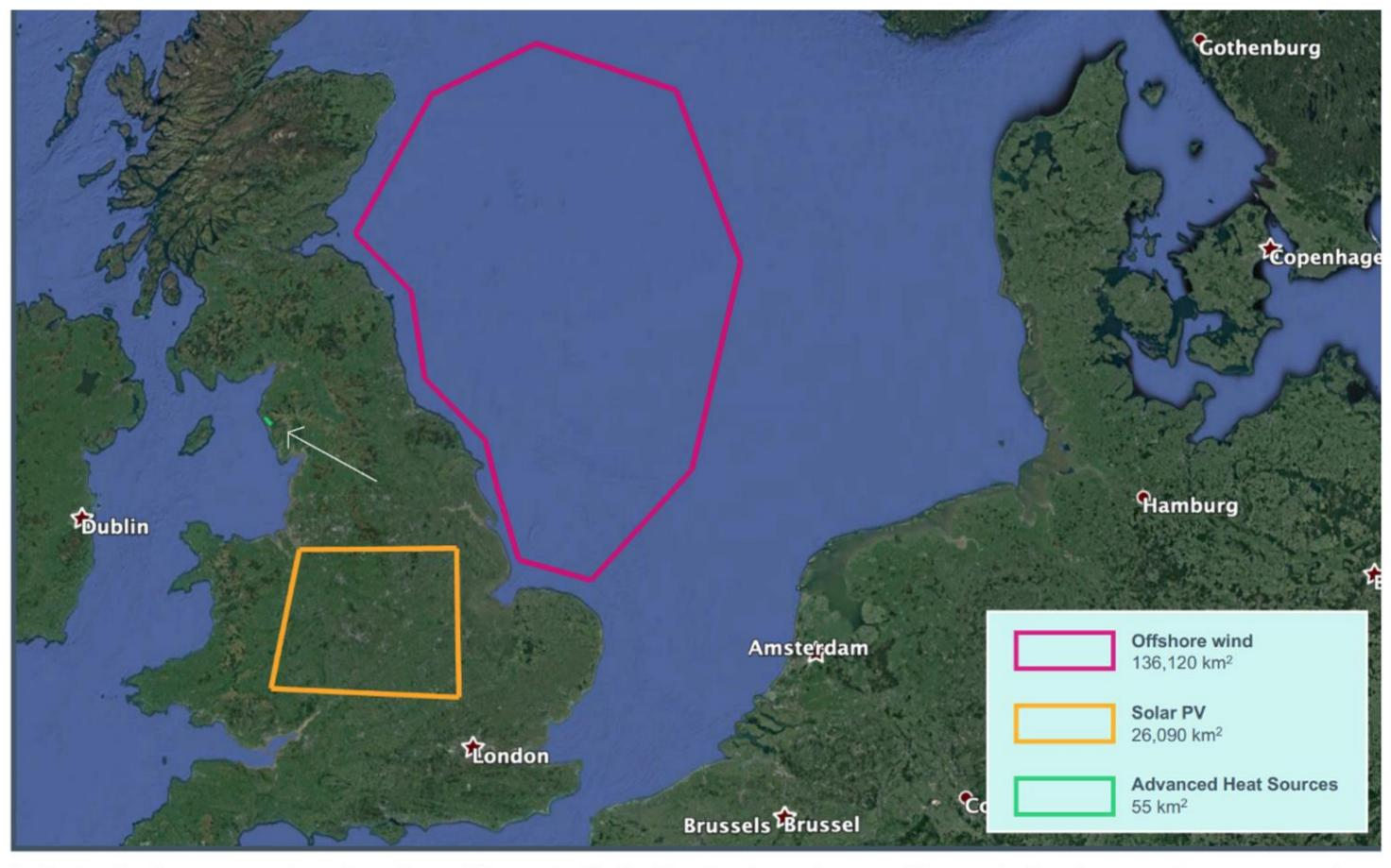
Comparing area required to replace the UK's current oil consumption with hydrogen generated from either wind, solar, or advanced heat sources.
