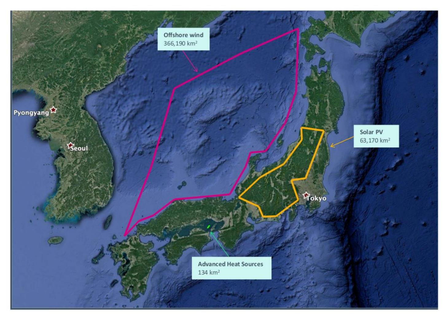
Comparing the total area required to replace Japan's current oil consumption with hydrogen generated from either wind, solar, or advanced heat sources
