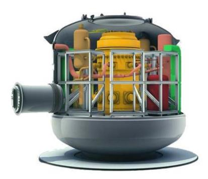
Among the different concepts, the so-called integrated designs, in which steam generators and pressurizer are located inside the pressure vessel, are the most promising ones. They indeed offer simpler design and inherent safety advantages. Furthermore, these designs rely on passive systems for residual heat removal during hypothetical loss of coolant accidents or station black out scenarios.
