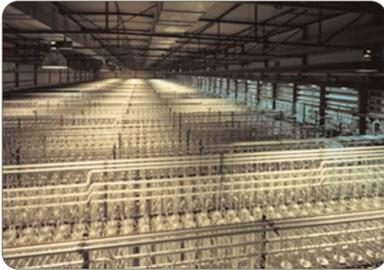
Uranium enrichment based on centrifuge technology
